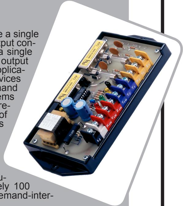
High output red, yellow and green LED lamps indicate the systems status at all times thus allowing a rapid visual check of the system's performance without requiring any additional test equipment. The IPR-1's input and output circuit's terminal strip is color coded for error free wiring in the field. Each "K" lead of the IPR-1's outputs is fused to prevent damage to the relays under almost any conditions a user might cause such as excessive current, incorrect wiring, etc.
